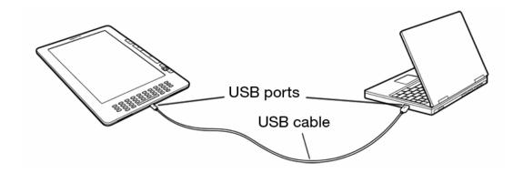
When you are connected to your PC, your Kindle will go into USB drive mode and its battery will be recharged by the computer. Your Whispernet service is temporarily shut off and you will not receive any of your subscriptions while in this mode. Also, your Kindle is not usable as a reading device while you are in USB drive mode, but will return right to where you were when you un-mount the device from your computer.
